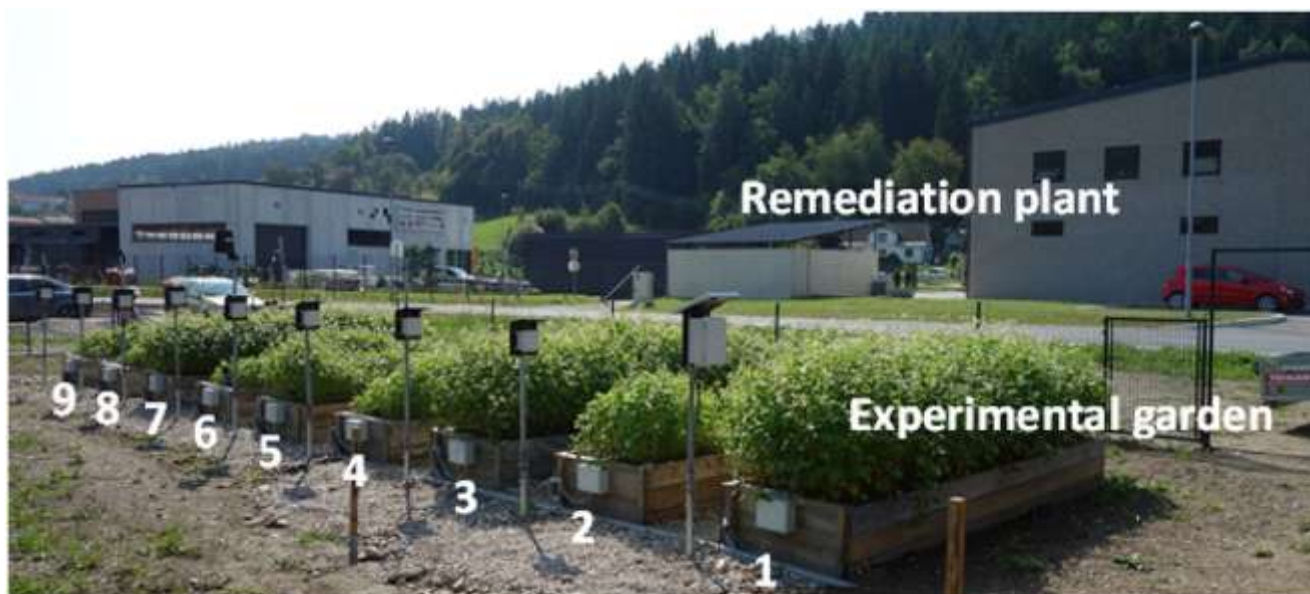
Figure 7.4- The experimental vegetable garden with nine raised beds constructed as lysimeters in the vicinity of demonstrational remediation plant with ReSoil® technology.
