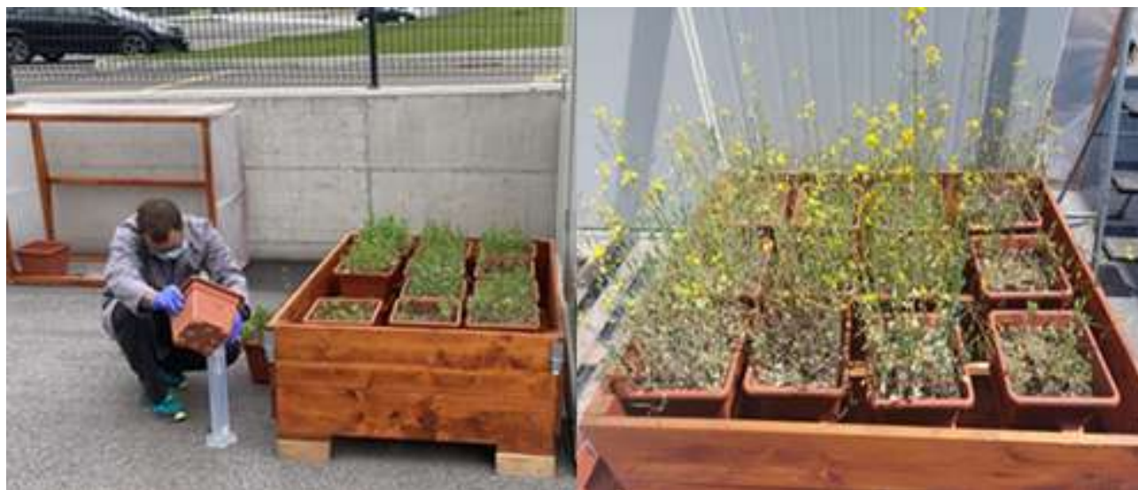
Figure 7.6- The collection of leachates and phytomanagement of ReSoil® remediated soil with rapeseed ( Brassica napus ).
